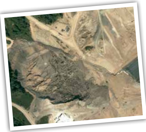
An aerial view of the slide. The higher elevation is lower center; the slide area is from that point to the upper left. Big Run Landfill photo
